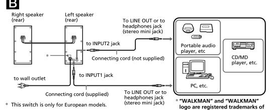
Sony Corporation. About the INPUT 1 and INPUT 2 jacks Connect to a portable audio player, PC, etc., with a headphones jack or LINE OUT jack. When the component has both a headphones jack and a LINE OUT jack, connect to the LINE OUT jack of this system. If you connect to the headphones jack of this system, turn down the connected component volume level to prevent audio
