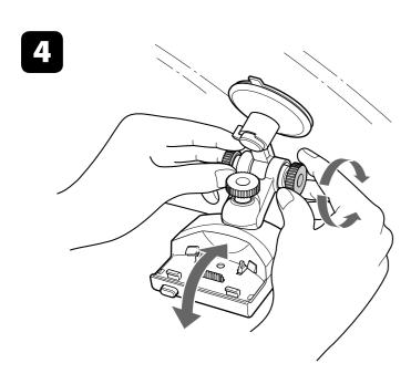
**Note**If you are concerned about car vibration and want to stabilize the unit, cut the supplied pad **G** to the appropriate size and attach it to the cradle bottom, to sit between the cradle and dashboard.
