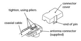
**3** Connect the antenna connector to the VHF/UHF antenna terminal.
