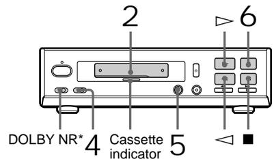
\* This tape deck is equipped with the Dolby B-type noise reduction system.
