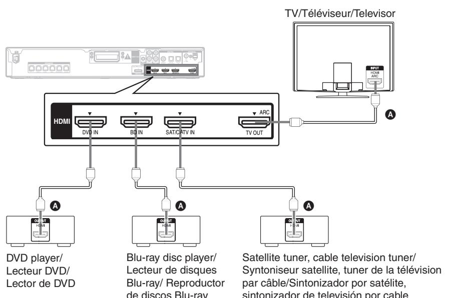
**A** HDMI cable (not supplied)/Câble HDMI (non fourni)/Cable HDMI (no suministrado)
