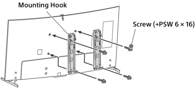
**3** Make sure that the wall has enough space for the TV and is capable of supporting a weight of at least four times that of the TV. Refer to the following table on installing the TV to the wall. See page 18-21 (Specifications) for the TV's weight.
