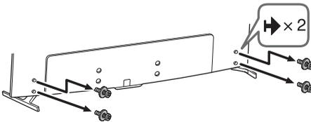
**6** Install the TV to the Base. Refer to "5" of Installation Guide and "Installing the TV to the Wall" of Operating Instructions supplied with the Wall-Mount Bracket.
