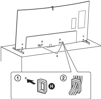
\* Location of cable clamer when the Table-Top Stand is attached to middle position.
