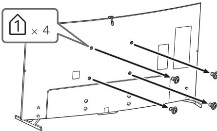
**2** Attach the Mounting Hook using the four screws supplied with the Wall-Mount Bracket.
