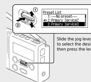
Slide the jog lever up or down to select the desired station (1), then press the lever (2).
