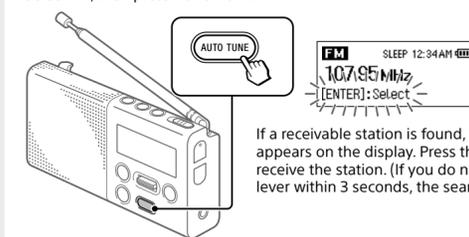
If a receivable station is found, "[ENTER]:Select" appears on the display. Press the jog lever to receive the station. (If you do not press the jog lever within 3 seconds, the search will restart.)
