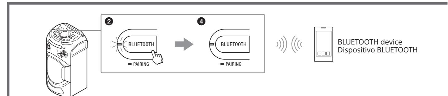
Be sure to place the BLUETOOTH device within 1 meter (3.3 feet) from the unit.
