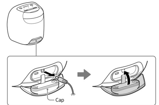
\*3 If a AC power cord is supplied, the shape of the plug on the AC adaptor and the connection method differ. According your country or region, connect the AC power cord to the AC adaptor.
