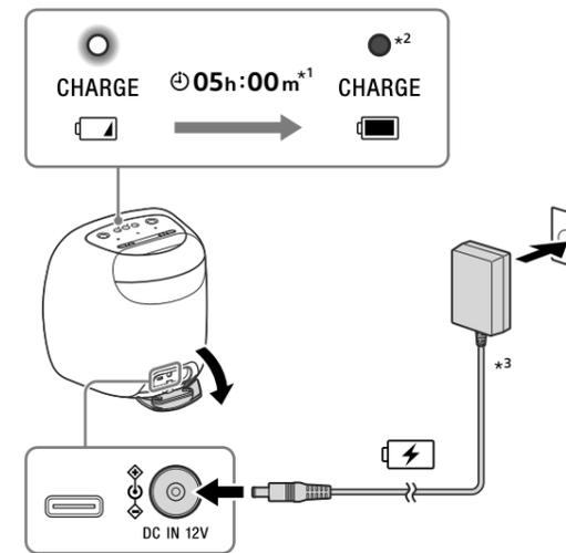
\*1 Time that is required to charge the empty built-in battery to its full capacity when the unit turns off.
