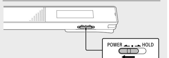
Slide and hold the POWER+HOLD switch in the direction of "POWER" until the window display appears. To turn the power off, slide the POWER+HOLD switch to "POWER" and hold it until "Power Off" appears on the display window.
