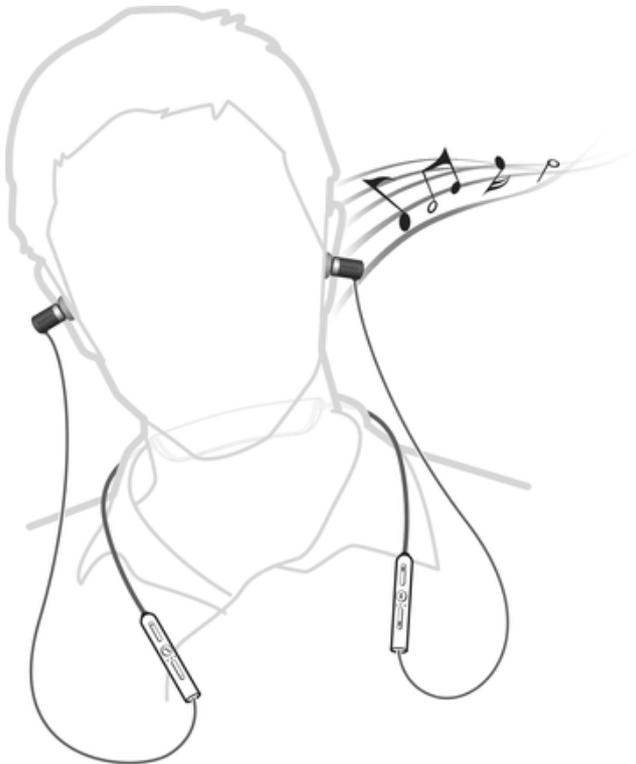
To get the best performance from your headset when using it outdoors, it is recommended that you carry the device that you have paired with the headset on the same side of your body as the antenna of the headset unit.
