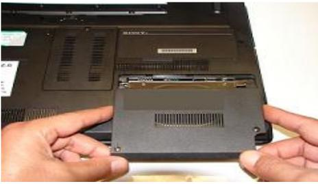
**Step 4.** Remove HDD access cover and set aside.
