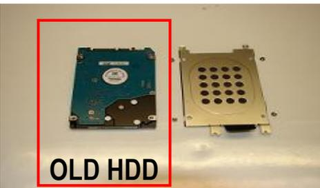
**Step 10.** All (4) screws and bracket should now be removed from old HDD. Set old HDD aside.
