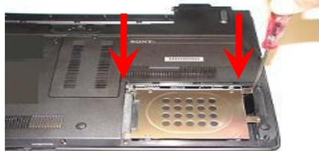
**Step 16.** Reinstall the (2) screws previously removed.
