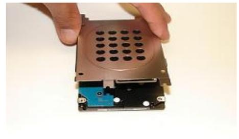
**Step 12.** Place the HDD bracket over the new HDD.
