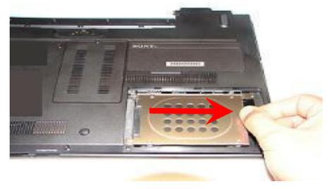
**Step 6.** Locate the black plastic tab on the hard drive assembly and gently pull the original hard drive to the right to disconnect from connector.
