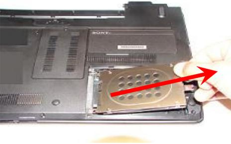
**Step 7.** Once the hard drive assembly is disconnected from the connector carefully lift the hard drive assembly to remove from hard drive bay.
