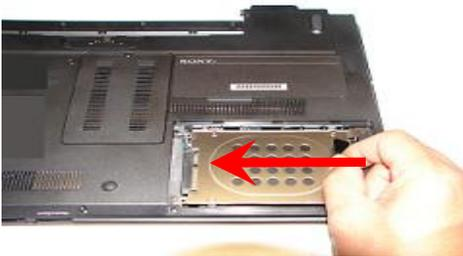
**Step 15.** Hold plastic tab and slide HDD to the left, carefully reconnecting the hard drive to the connector.
