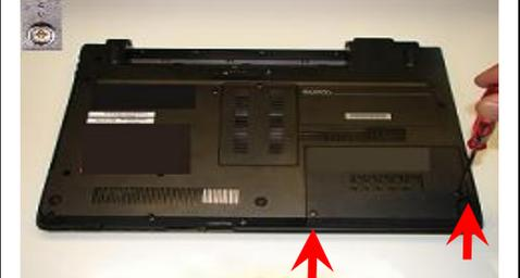
**Step 17.** Reinstall the hard drive cover and install the (2) screws previously removed.
