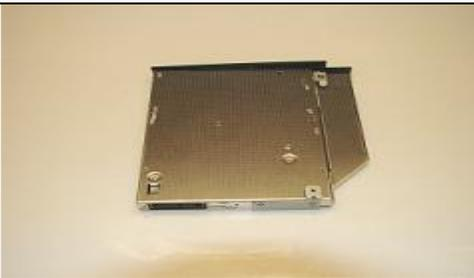
**Note!** Flat surface of bracket should sit flush with silver side of ODD.
