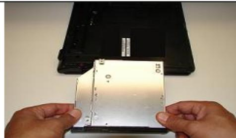
**Step 15.** To install the new drive, hold the optical drive by the edges and align it with the bay opening.
