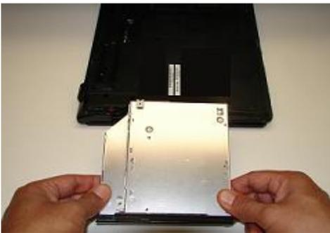
**Step 7.** Carefully remove the ODD assembly.
