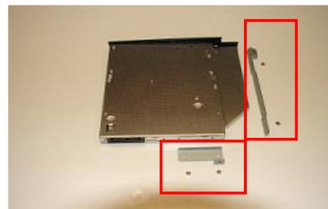
**Step 10.** Bracket & screws should now be removed. Please arrange the bracket & screws as shown above. Set old ODD aside.
