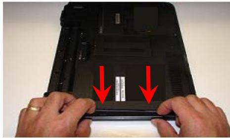
**Step 5.** To initiate the removal of the optical drive, slightly pull the optical drive door as shown in the picture. Slight force may be needed to disconnect drive from connector.
