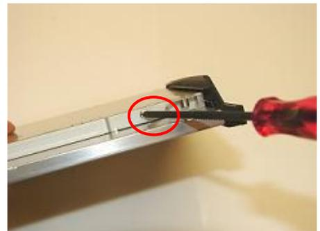
**Step 9.** Firmly but carefully hold the ODD. Remove the screws & brackets and set them aside. The screws & brackets will be used on the new ODD provided.
