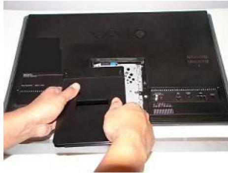
**Step 5.** Set HDD cover aside once removed.
