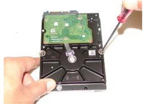
**Step 14.** Remove the (2) screws to be used on new HDD.
