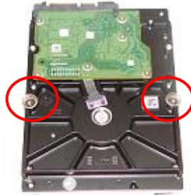
**Step 13.** After the HDD is completely removed from bracket, identify the (2) screws with springs.
