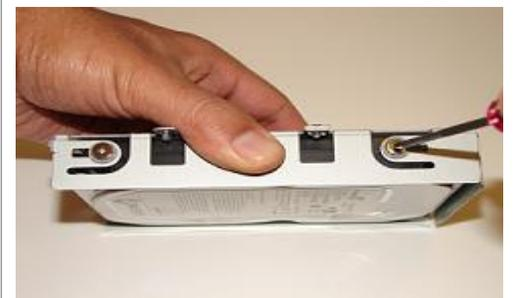
**Step 11.** Holding the edge of the HDD, remove each screw and set the screw aside. **These screws will be used to mount the HDD bracket onto the new HDD.e.**
