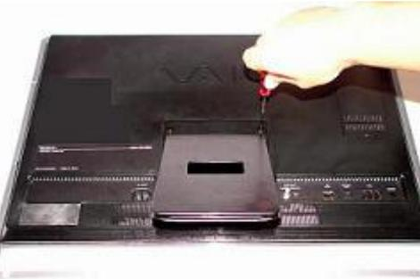
**Step 23.** Re-install the (4) screws previously removed.
