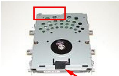
**NOTE!** Proper mounting of HDD bracket can be verified with the HDD connectors appearing opposite the bracket tabs.
