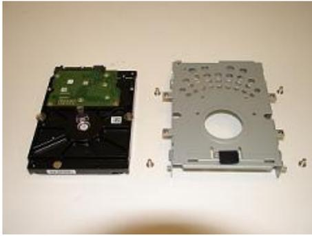
**Step 12.** All (4) screws and bracket should now be removed from old HDD.
