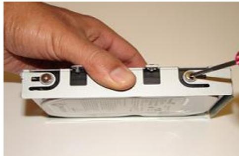
**Step 18.** Re-install the (2) screws with springs previously removed.
