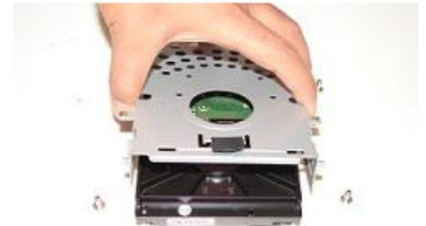
**Step 17.** Place the HDD bracket over the new HDD.
