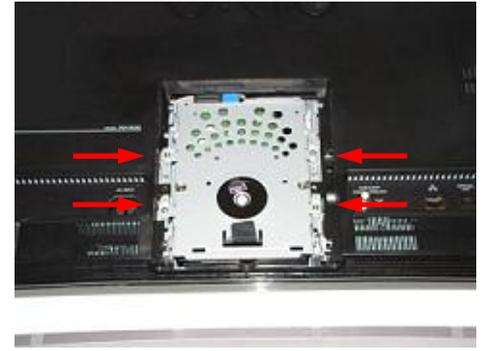
**Step 6.** Identify the (4) screws securing the HDD to the computer.
