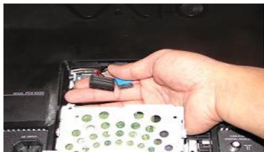
**Step 9.** Remove connectors before attempting to completely remove HDD assembly.
