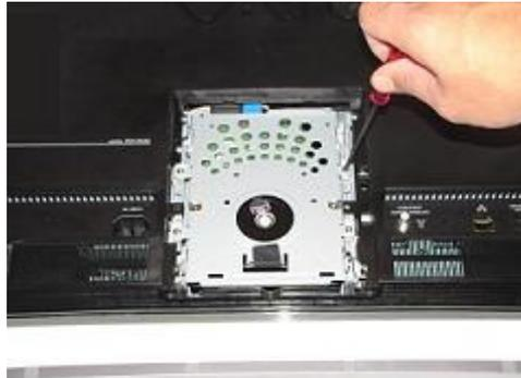
**Step 21.** Once assembly is properly aligned re-connect the (4) screws previously loosened.
