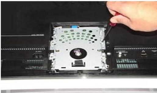
**Step 7.** Using the included magnetic screwdriver, loosen the (4) screws securing the HDD Assembly.
