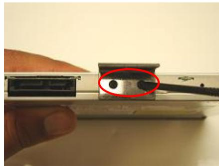
**Step 8.** Remove the screws & bracket. **Put the ODD Brackets and screws aside for transfer to the new ODD.**
