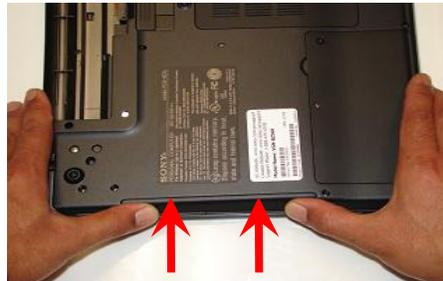
**Step 15.** Make sure the new ODD is seated flush on the edge of the computer.
