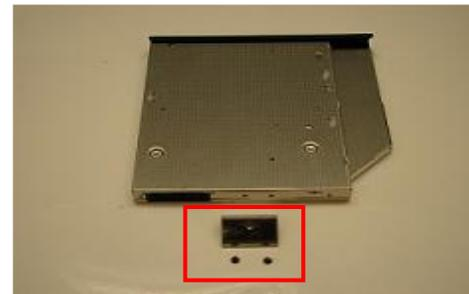
**Step 9.** Arrange the brackets & screws as shown above. Set the old ODD aside.
