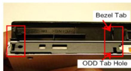
**NOTE:** Identify tabs on the bezel and tab holes located on the ODD.
