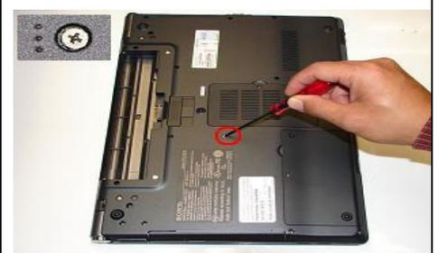
**Step 16.** Reinstall the one (1) ODD Bay screw to secure the ODD Drive Bay.
