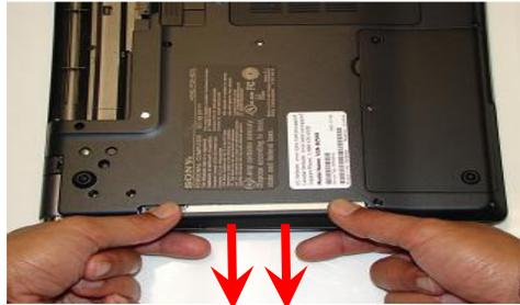
**Step 5.** Insert your fingers in the space between the ODD and the unit. Gently pull towards the left to remove the ODD.
