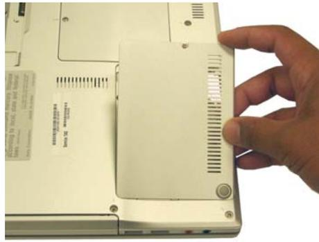
**Step 5.** To remove the HDD access cover, start by lifting from the side where the screw held it in place.
