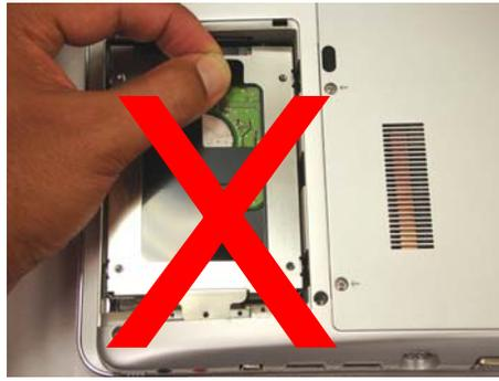
**CAUTION:** Do not pull the plastic tab before releasing the hard drive from the connector!
