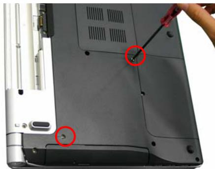
**Step 10.** Reinstall the two screws previously removed.
