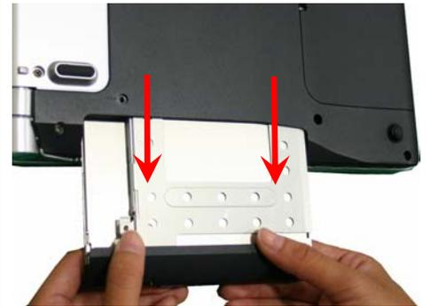
**Step 6.** With even force, slide out the ODD as shown. Some force may be required to unlock the ODD from the connector.
