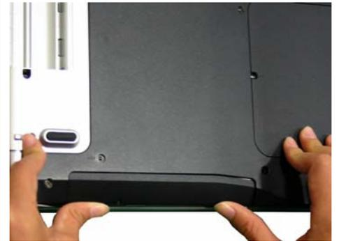
**Step 9.** Make sure the new ODD Bay is seated flush on the edge of the computer.
