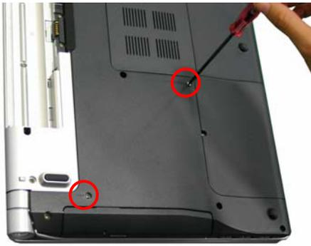
**Step 4.** Using the enclosed magnetic screwdriver, remove the two screws securing the ODD Bay.
