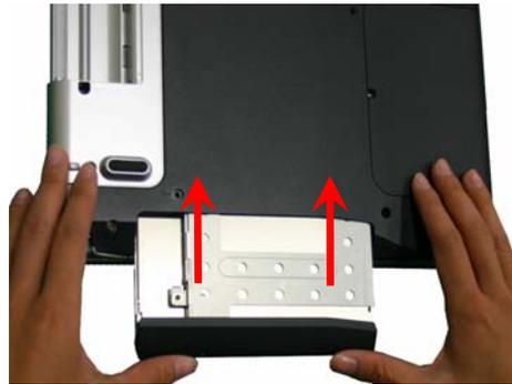
**Step 8.** With an even force slide in the new ODD Bay.
