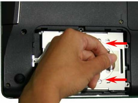
**Step 8.** To detach the old HDD from the connector, slowly pull the clear plastic tab in the direction shown. Some force may be needed to unlock the HDD from the connector.
