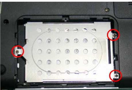
**Step 11.** Re-install the three (3) screws holding the HDD assembly in place.
