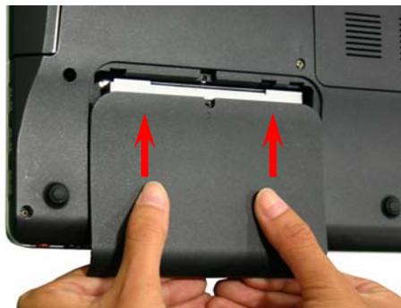
**Step 12.** Re-attach the HDD access cover by sliding it in the direction shown in the picture. Secure the HDD Bay access door with the one (1) screw that was previously removed.
