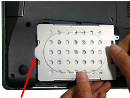
Insert HDD Housing Tab in Slot
