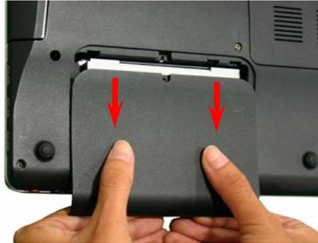
**Step 6.** Carefully remove the HDD Bay Access door by sliding it in the direction shown in the picture.
