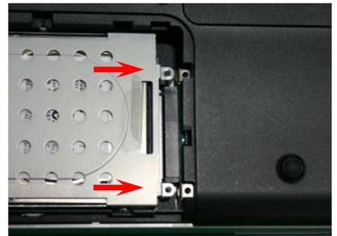
**Step 10. Attach the HDD to the Connector.**
