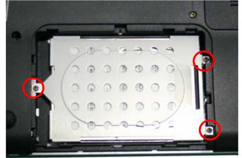
**Step 7.** Locate the three (3) screws securing the HDD assembly and remove them accordingly.
