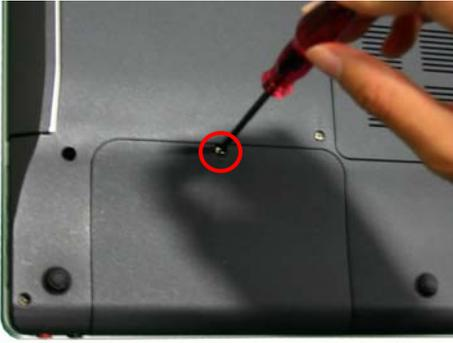
**Step 5.** Using the enclosed magnetic screwdriver, remove the one (1) screw securing the HDD Bay Access door.
