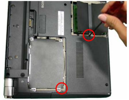
**Step 6.** Remove the two (2) screws shown in the picture. These are the screws that secure the ODD in place.
