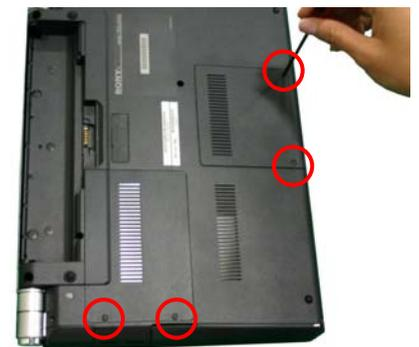
**Step 12.** Reinstall the Memory and HDD access covers.
