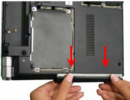
**Step 7.** To initiate the removal of the ODD Bay, pull slightly the ODD door as shown in the picture.
