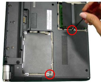
**Step 11.** Reinstall the two (2) screws securing the ODD in place.
