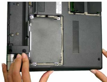
**Step 10.** Make sure the new ODD Bay is seated flush on the edge of the computer.
