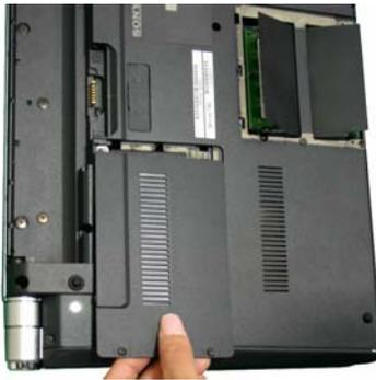
**Step 5.** Remove the Memory and HDD access covers. Start by lifting from the side where the screws held them in place.
