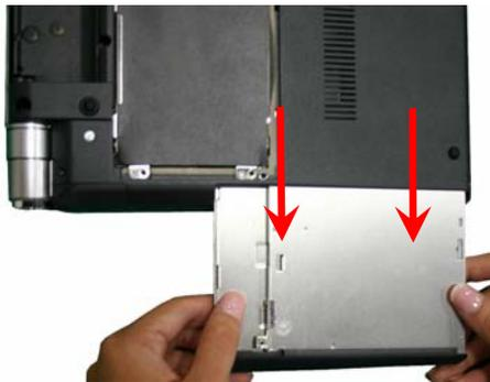
**Step 8.** With even force, slide out the ODD as shown. Some force may be required to unlock the ODD from the connector.
