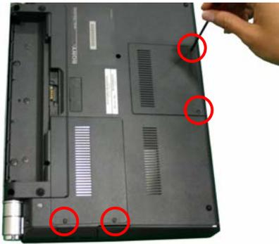
**Step 4.** Using the magnetic screwdriver, loosen the four screws securing the Memory and HDD access covers.
