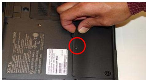
**Step 11.** Reinstall the hard drive cover and tighten the screw previously loosened.
