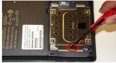
**Step 5.** Using the enclosed magnetic screwdriver, **remove** the one (1) screw securing the hard drive assembly.
