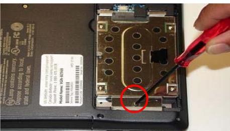
**Step 10.** Reinstall the one screw previously removed.
