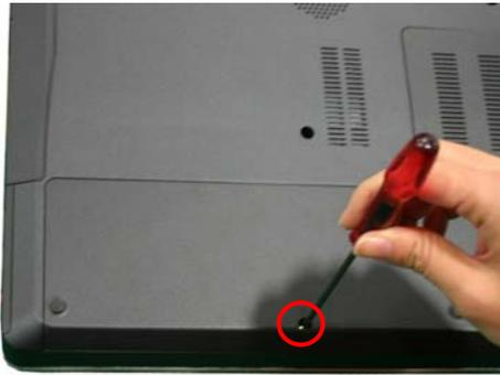
**Step 5.** Using the enclosed magnetic screwdriver, remove the screw securing the hard disk drive access cover.
