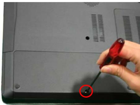
**Step 12.** Re-attach the HDD access cover and secure it with the screw shown in the picture.
