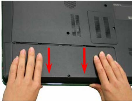
**Step 6.** Remove the HDD access cover by sliding it in the direction of the arrows shown above.
