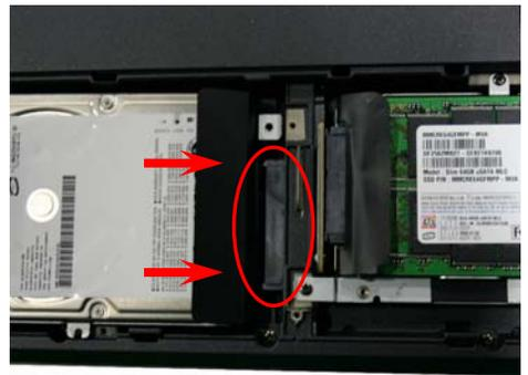
**Step 10.** Attach the drive to the HDD connector by moving the new HDD assembly in the direction of the arrows shown in the picture.
