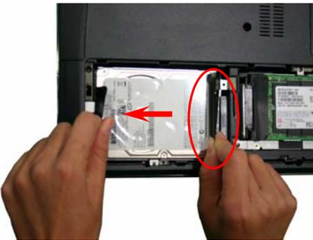
**Step 8.** To remove the drive, carefully detach the HDD from the connector in the direction shown. Some force may be needed to unlock the HDD from the connector. Lift the drive by holding on the black plastic tabs to remove it completely.
