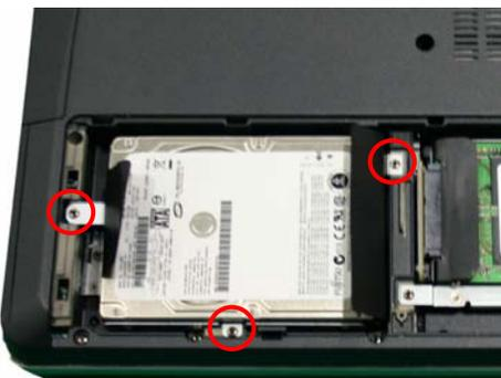
**Step 11.** Reinstall the three (3) previously removed screws to secure the HDD bay in place.
