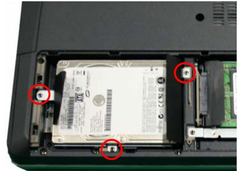
**Step 7.** Using the enclosed magnetic screwdriver, remove the three (3) screws securing the HDD assembly.
