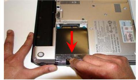
**(HDD must be disconnected)**
