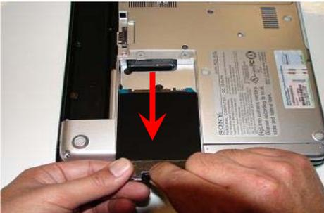
**Step 7.** Once the hard drive assembly is disconnected from the connector carefully lift the hard drive assembly to remove from hard drive bay.
