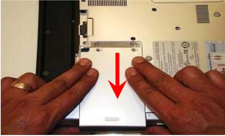
**Step 4.** To remove the hard drive access cover slide the cover as shown above .
