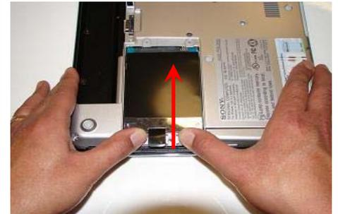
**Step 9.** Once hard drive is properly sitting its bay, carefully re-connect the hard drive to the connector by sliding the hard drive in the direction shown above.
