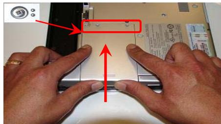
**Step 11.** Reinstall the hard drive cover by sliding the cover in the direction shown above and tighten the two (2) screws previously removed.
