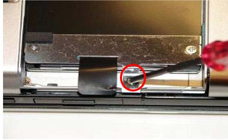
**Step 5.** Using the enclosed magnetic screwdriver, **remove** the one (1) screw securing the hard drive assembly.
