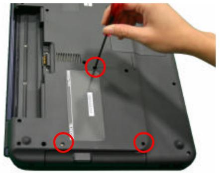
**Step 9.** Secure the new ODD by re-installing the three (3) screws previously removed.
