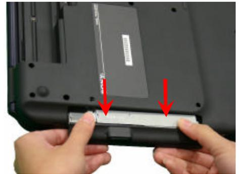
**Step 6.** With even force, slide out the ODD as shown. Some force may be required to unlock the ODD from the connector.
