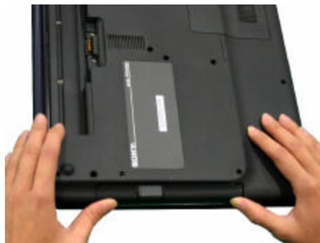
**Step 8.** Make sure the new ODD is seated flush on the edge of the computer.
