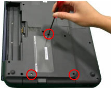
**Step 4.** Using the magnetic screwdriver, remove the three (3) screws securing the ODD.
