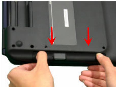
**Step 5.** To initiate the removal of the ODD, pull slightly the ODD door as shown in the picture.
