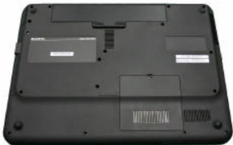
**Step 10.** Reinstall the battery pack. Return the old ODD to Sony following the included shipping instructions.
