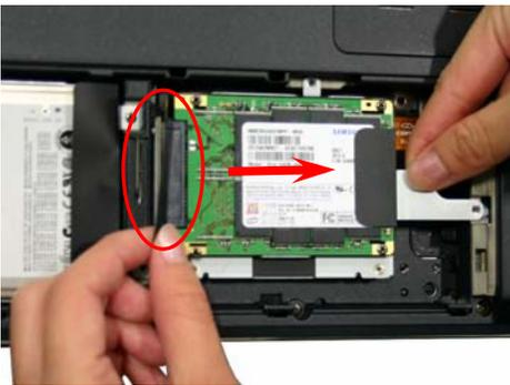
**Step 8.** To remove the drive(s), carefully detach the SSD from the connector in the direction shown. Some force may be needed to unlock the SSD assembly from the connector. Remove the drive by holding on the black plastic tab and housing.
