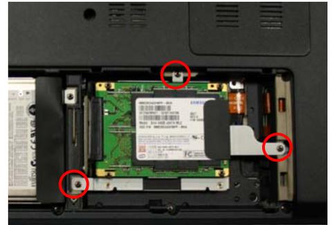
**Step 7.** Using the enclosed magnetic screwdriver, remove the three (3) screws securing the SSD assembly.
