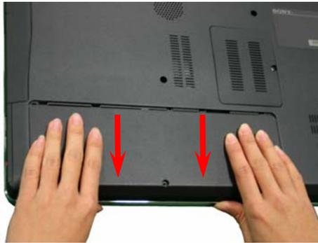
**Step 6.** Remove the SSD/HDD access cover by sliding it in the direction of the arrows shown above.
