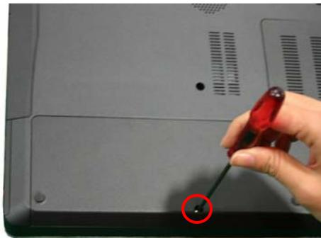
**Step 12.** Re-attach the SSD/HDD access cover and secure it with the screw shown in the picture.
