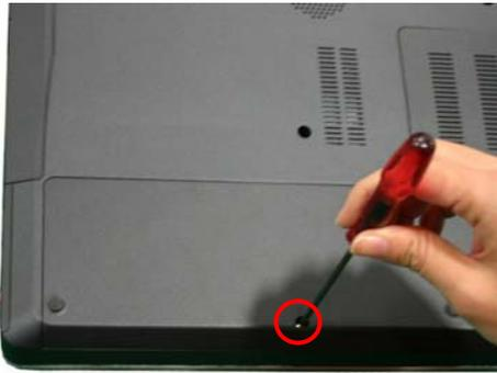
**Step 5.** Using the enclosed magnetic screwdriver, remove the screw securing the SSD/HDD access cover.
