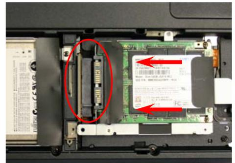
**Step 10.** Attach the drive(s) to the SSD connector by moving the new SSD assembly in the direction of the arrows shown in the picture.
