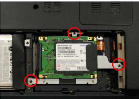
**Step 11.** Reinstall the three (3) previously removed screws to secure the SSD assembly in place.
