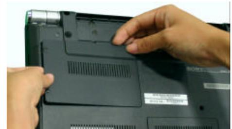
To remove the HDD access cover, start by lifting from the side where the screws held it in place.
