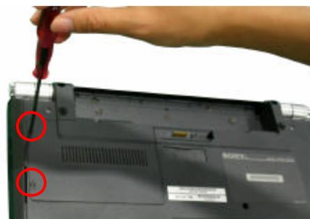
**Step 12.** Re-attach the HDD access cover and secure it with the two (2) screws shown in the picture.
