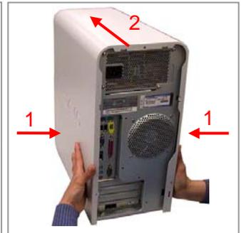
**Step 9.** Lower the cover onto the unit, Ensure that tabs on the bottom edge into the base of your computer. Compress both sides of the cover and push forward while holding the front of your computer. Reinstall the three (3) screws removed in step 1.
