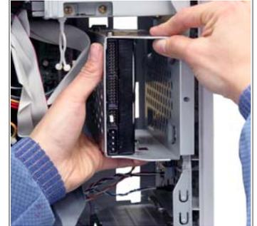
**Step 5.** Using the enclosed magnetic screwdriver, remove the marked screw as shown on the picture. With one hand hold the bracket enclosure while pulling the complete assembly out of the unit.
