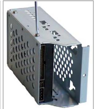
**Step 7.** Slide New Hard drive inside bracket with all holes in alignment. Reinstall the four (4) screws previously removed, securing new drive into the bracket.
