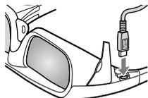
5 Plug the other end of the USB charging cable into the USB port on the computer.
