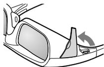
4 Plug one end of the supplied USB charging cable into the connector for charge on the 3D glasses.
