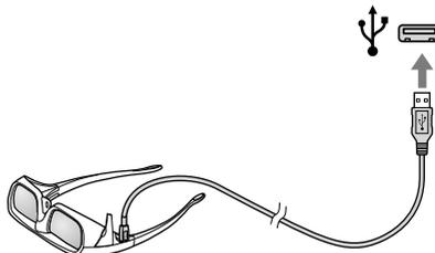
The battery starts charging and the yellow LED indicator light on the 3D glasses turns on.
