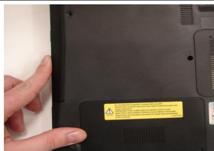
**Step 15.** Make sure the new ODD is seated flush on the edge of the computer.
