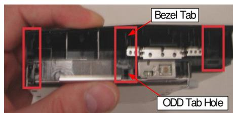
**NOTE:** Identify tabs on the bezel and tab holes located on the ODD.
