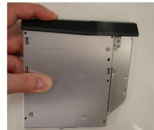
**Step 11.** Align the tabs on the bezel with the tab holes located on the ODD. Carefully press the bezel into place.
