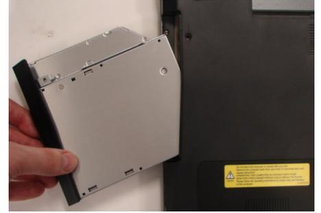
**Step 6.** Carefully remove the ODD assembly from the unit.
