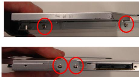
**Step 8.** Remove the screws & brackets. **Put the ODD Brackets and screws aside for transfer to the new ODD.**
