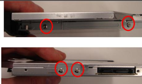
**Step 13.** Using the ODD Screws, install the ODD Brackets onto the new ODD.
