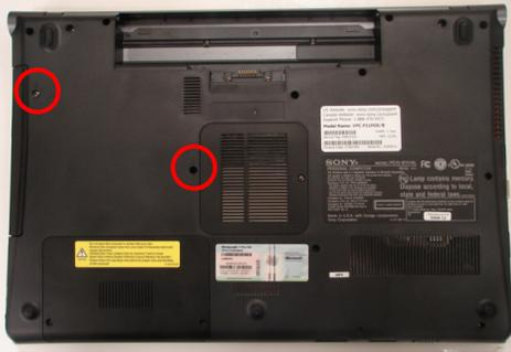
**Step 4.** Using the enclosed magnetic screwdriver, remove the two (2) screws securing the ODD Bay. **Put aside the ODD Bay screws to re-secure the ODD Bay later in the procedure.**
