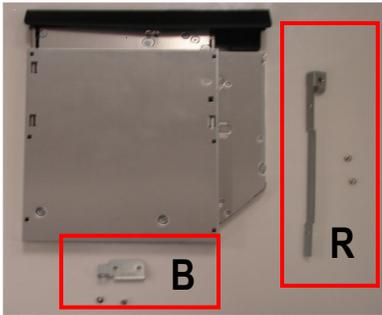
**Step 12.** Position the new ODD (Label side down) and identify the correct bracket with the corresponding ODD side (as shown). Take note of the different shapes for each bracket and the proper alignment of the screw holes.
