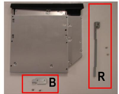
**Step 9.** Arrange the brackets & screws as shown above. Set the old ODD aside.
