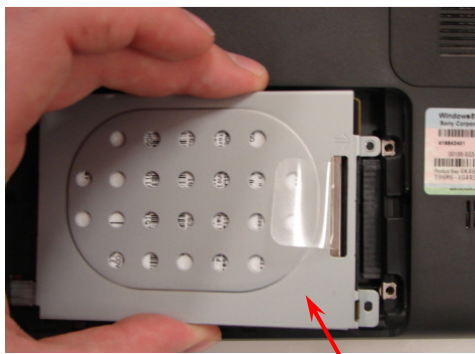
Step 7. Carefully lift the Hard Drive from the unit to remove. Lift To Remove
