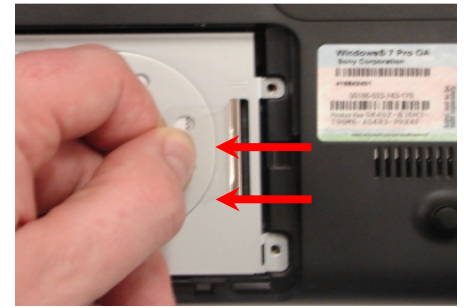
Step 6. Disconnect the Hard Drive by pulling the clear plastic tab to the left.
