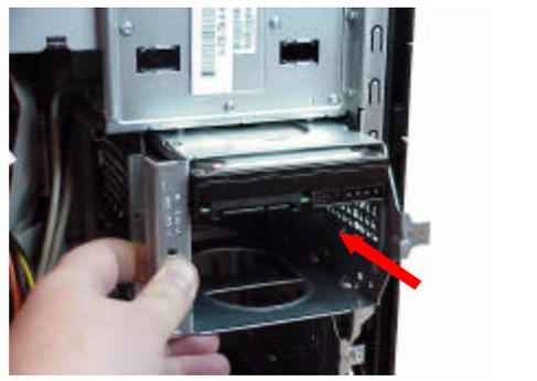
**Step 10.** Slide the hard drive bracket enclosures back inside the unit, making sure all holes are lined up.
