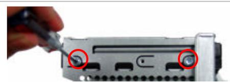
**Step 9.** Reinstall the four (4) previously removed screws into indicated positions on both sides of the bracket. **IMPORTANT!** Do not over tighten the screws!
