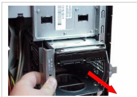
**Step 4.** Pull the hard drive bracket enclosure from the unit in the direction of the arrow.
