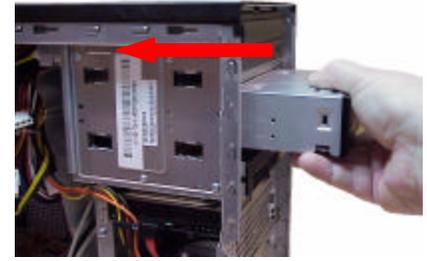
**Step 7.** Carefully slide the new optical drive into the newly vacant space in the chassis, making sure the screw holes are aligned.
