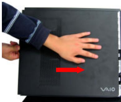
**Step 11.** Reinstall the left chassis cover panel in the direction of arrow. Then using the enclosed magnetic screwdriver, reinstall the two (2) previously removed screws. **IMPORTANT!** Do not over tighten the screws! Return the original optical disk drive to Sony following the included shipping instructions
