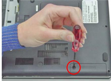
**Step 5.** Remove the HDD Bay.
