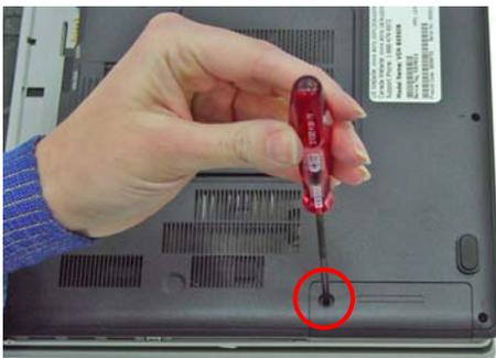
**Step 10.** Reinstall the one (1) screw previously removed.
