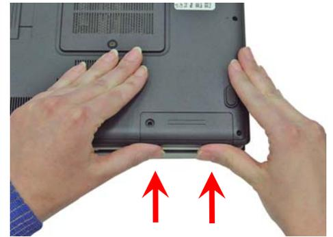
**Step 9.** With an even force slide in the new HDD Bay.
