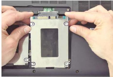
**Step 8.** Gently pull out the original HDD away from the computer as shown.
