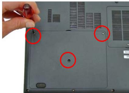
**Step 10.** Reinstall the three (3) screws previously removed.
