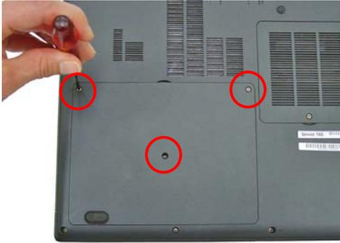
**Step 4.** Using enclosed magnetic screwdriver, loosen up the three (3) screws securing the hard drive access door. Gently remove the access door at an angle.
