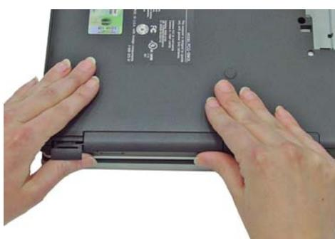
**Step 11.** Make sure the new ODD Bay is seating flush on the edge of the computer.
