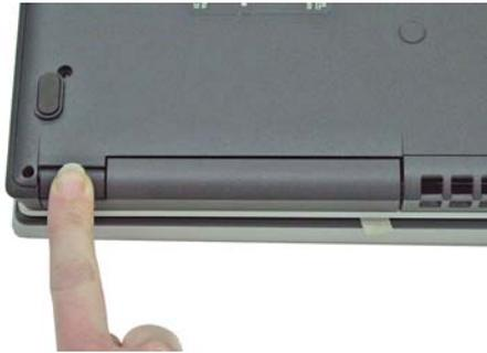
**Step 5.** Unlock the ODD Latch.
