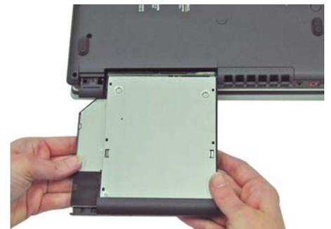
**Step 9.** Install New ODD Bay. Hold the new ODD Bay by the edges and align it with the opening.
