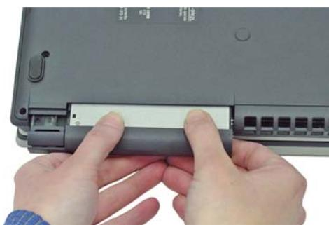
**Step 8.** Remove completely the ODD Bay.
