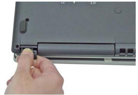
**Step 6.** To initiate the removal of the ODD Bay, pull slightly the ODD latch as shown.
