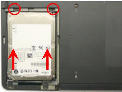
**Step 9.** Align the HDD with the connector and with even force push in the new HDD. Reinstall the two (2) previously removed screws.
