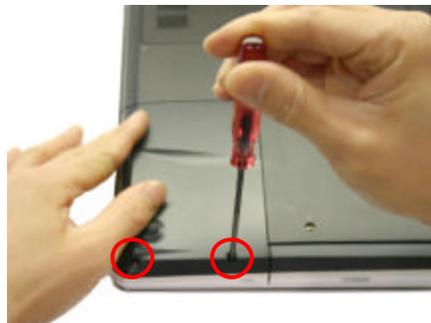
**Step 10.** Reinstall the HDD access door previously removed. Align the access door notch to avoid damage.
