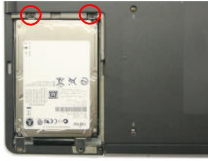
**Step 5.** Using the enclosed magnetic screwdriver, remove the two (2) screws as indicated in the picture.
