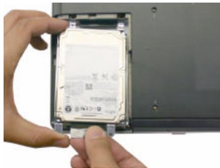
**Step 7.** Gently pull out the original HDD away from the computer as shown.
