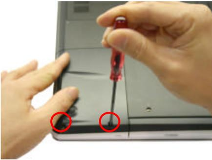
**Step 4.** Using the enclosed magnetic screwdriver, loosen the two (2) screws securing the hard disk drive access door. Gently remove the access door at an angle to avoid damaging the notch.
