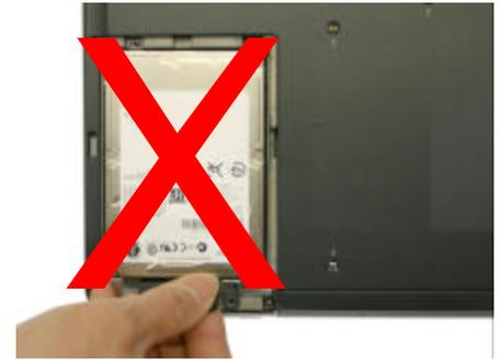
**CAUTION:** Do not pull the plastic tab upwards before releasing the hard drive from the connector!
