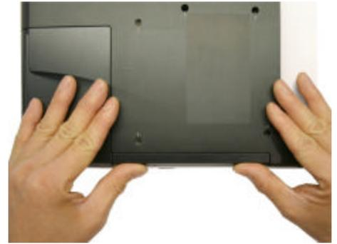
**Step 9.** Make sure the new ODD Bay is seating flush on the edge of the computer.
