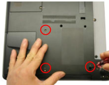
**Step 11.** Reinstall the three (3) previously removed screws.
