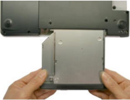
**Step 7.** Hold the new ODD Bay by the edges and align it with the opening. **IMPORTANT! Install the new ODD in the correct position.**
