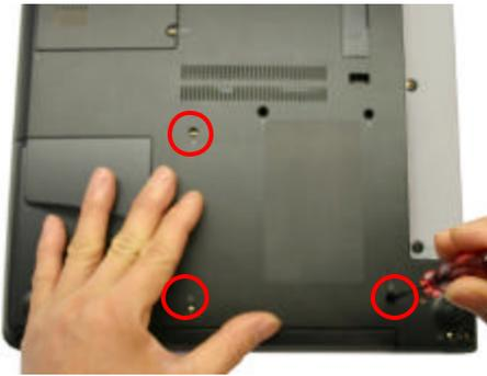
**Step 4.** Remove the ODD Bay. Using the enclosed magnetic screwdriver, loosen up the three (3) screws securing the ODD Bay.
