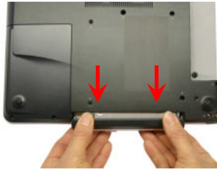
**Step 5.** To initiate the removal of the ODD Bay, pull slightly the ODD door as shown in the picture.
