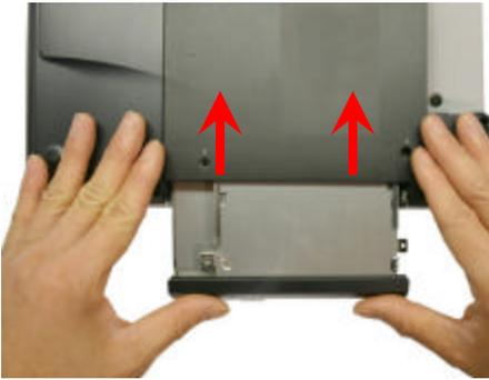
**Step 8.** With an even force slide in the new ODD Bay.
