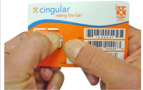
**Step 6.** Punch the SIM Card out of the card.
