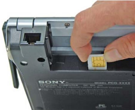
**Step 5.** Remove the SIM Card as shown.
