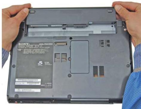
**Step 8.** Reinstall the Battery Pack.
