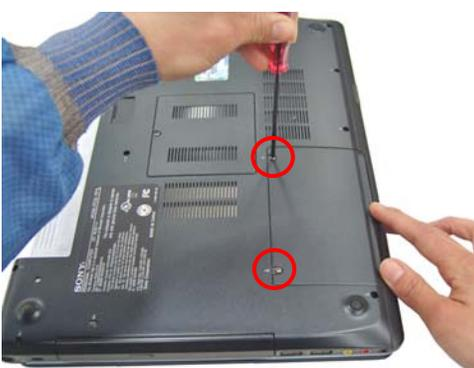
**Step 9.** Reinstall the HDD access door previously removed.
