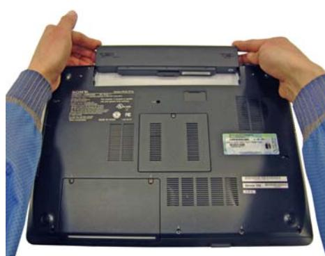
**Step 10.** Reinstall the Battery Pack. Reconnect the AC Adapter.
