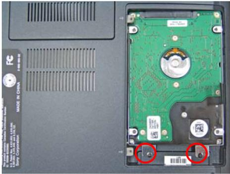
**Step 4.** Using the enclosed magnetic screwdriver, remove the two (2) screws as indicated in the picture.
