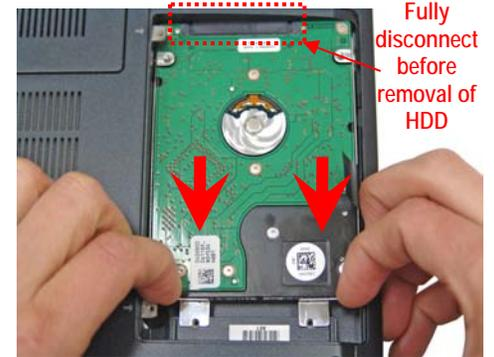
**Step 5.** With even force slide out the HDD as shown. Some force may be required to unlock the HDD from the connector.
