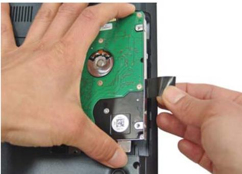
**Step 6.** Gently pull out the original HDD away from the computer as shown.
