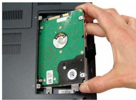
**Step 7.** Hold the new HDD by the edges and slide it inside the opening in an angle.
