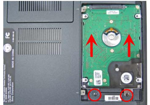
**Step 8.** Align the HDD with the connector and with even force push in the new HDD. Reinstall the two (2) previously removed screws.
