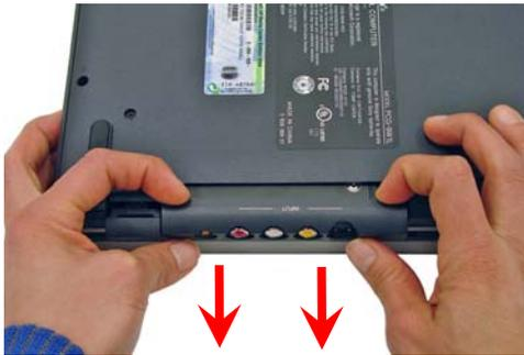
**Step 7.** Pull the TV Tuner Bay away from the computer as shown. Some force may be required to disconnect it.
