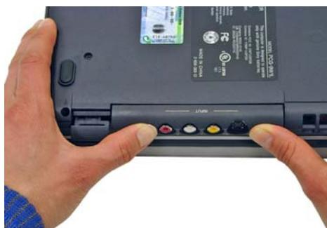
**Step 11.** Make sure the new TV Tuner Bay is seating flush on the edge of the computer.
