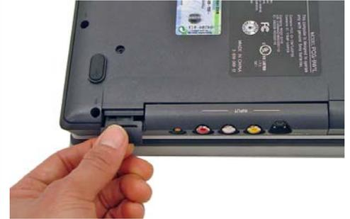
**Step 6.** To initiate the removal of the TV Tuner Bay, pull slightly the latch as shown.
