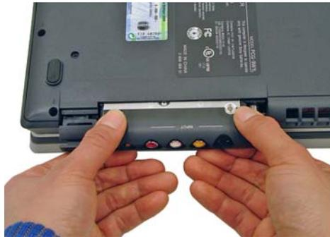
**Step 8.** Remove completely the TV Tuner Bay.
