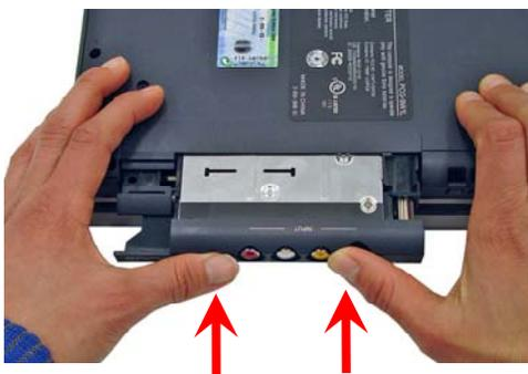
**Step 10.** With an even force slide in the new TV Tuner Bay.
