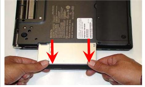
**Step 6.** With even force carefully remove the optical drive by pulling it away from the unit.
