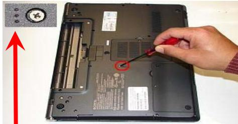
**Step 11.** Re-install the previously removed screw.
