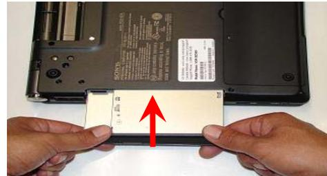
**Step 8.** Carefully slide the optical drive into the bay and back into place.
