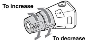
If you need to mount the rotary commander on the right hand side of the steering column, you can reverse the operative direction.
