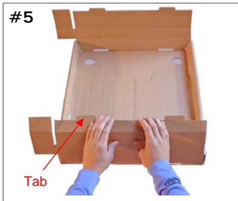
Turn tray, pre-fold and roll side flap towards inside of the tray (see photo #5), ensure that both tabs are fully inserted on open slots as shown on photo #6.
