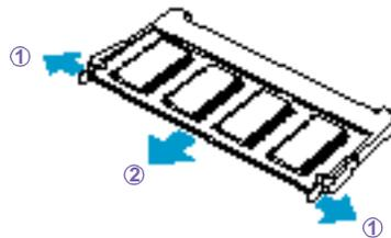
① Pull the tabs in the direction of the arrows. The memory module is released.
