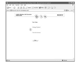
When you click "Execute Setup", the Wireless LAN Converter restarts. If the status indicator on the front panel of the Wireless Unit flashes slowly white, communication with the Access Point is established.
