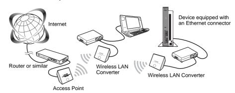
The Wireless LAN Converter also allows computers equipped with Wireless LAN Converters to communicate directly when using the Peer to Peer Network connection mode, without using a Wireless LAN Access Point.
