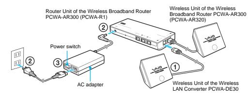
The connections above are used in configuring the Wireless LAN Converter with the Quick Setup switch. For details about connections to use the Wireless LAN Converter in wireless communication, see procedure 4.
