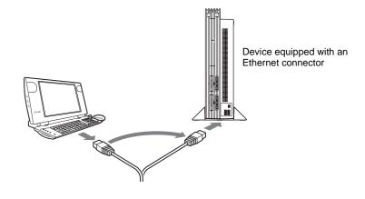
If you disconnect the Ethernet cable from the computer used for setup while it is still on, wait at least 10 seconds before connecting it to the wireless communication device
