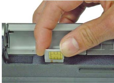
**Step 5.** Remove the SIM Card as shown.
