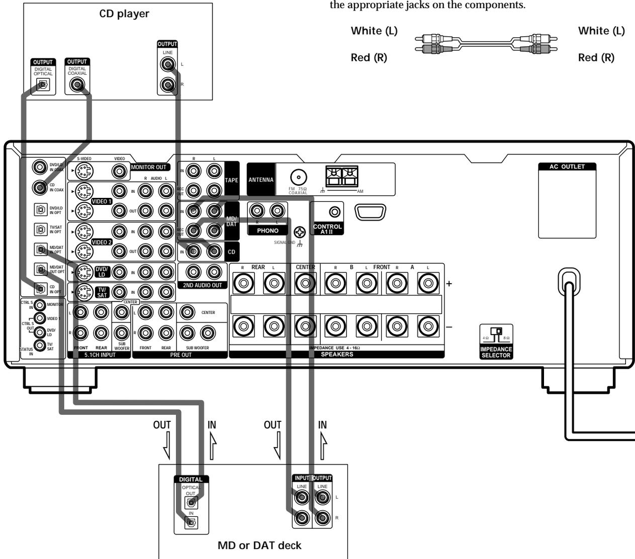
\* Make either coaxial or optical connections. We recommended making coaxial connections instead of optical connections.
