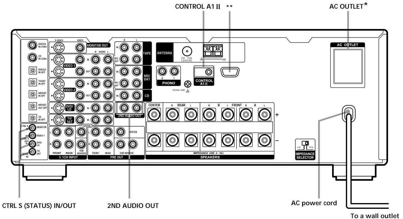
\* The configuration, shape, and number of AC outlets on the rear panel varies according to the model and country to which the receiver is shipped.
