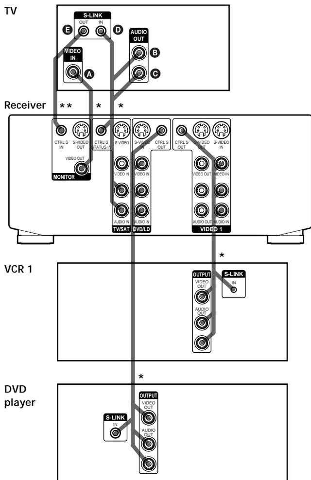
\* Audio/video/control S connecting cord (Pull the video cord away from the supplied audio/video/control S cable for connection **A**.)
