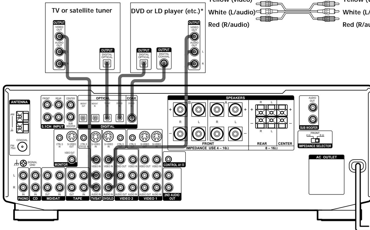
\* Make either coaxial or optical connections. We recommended making coaxial connections instead of optical connections.
