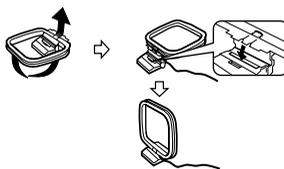
**4** Connect the AM loop antenna to the AM terminals on the back of this unit.
