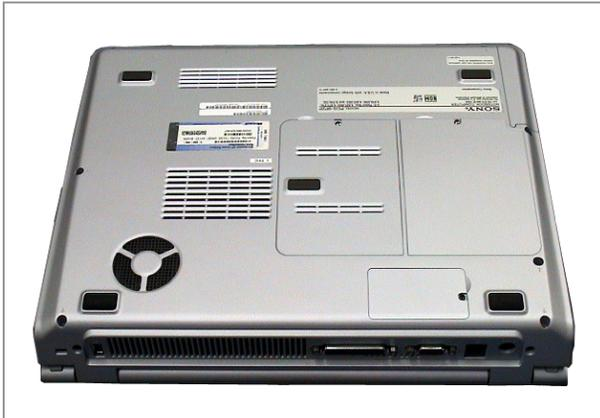
**Step 1.** To prevent any kind of cosmetic damages and scratches, place your PC upside down on top of a soft surface, with the ports facing you.
