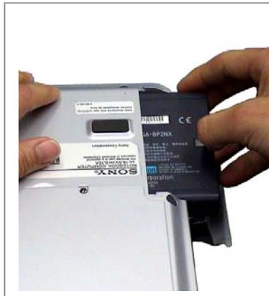
**Step 2. CAUTION!**
