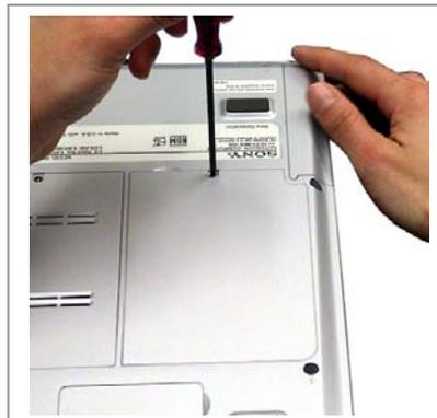
**Step 10.** Reinstall the hard drive access door and screw. Power on your computer and continue with the recovery process by following the instructions described on the back of the recovery disk's case.
