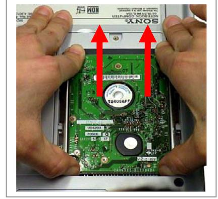
**Step 6.** Gently slide the drive in the direction of the arrows to release the pins from the socket.
