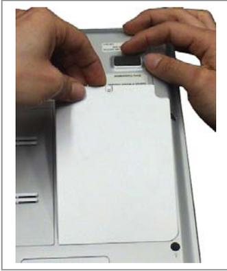
**Step 4.** Remove hard drive access door as shown and set aside.
