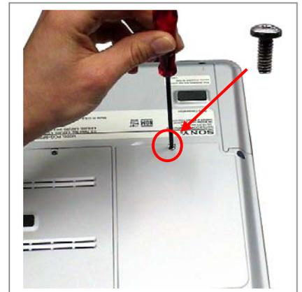
**Step 3.** Using the enclosed magnetic screwdriver, remove the marked screw and set aside.
