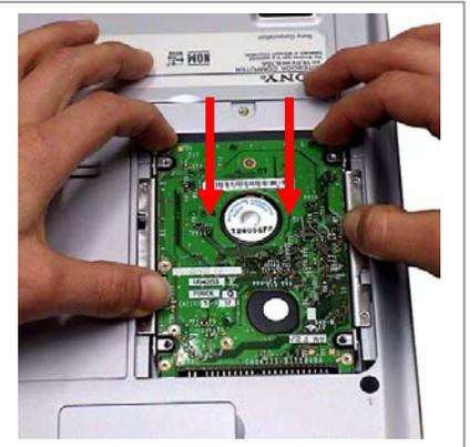
**Step 8.** Place the new drive flat in the opening. Slide the drive into position in the direction of the arrows, as shown above. Make sure both rows of pins have been inserted into the socket.
