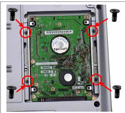
**Step 9.** Using the enclosed magnetic screwdriver, reinstall the four (4) previously removed screws. **CAUTION!** Be careful not to drop screws into the unit, and be careful to use the correct screws, as shown in the picture. Do not over tighten the screws!
